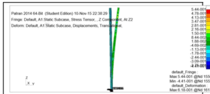
Fig4. Results showing the variation of longitudinal normal stress.
